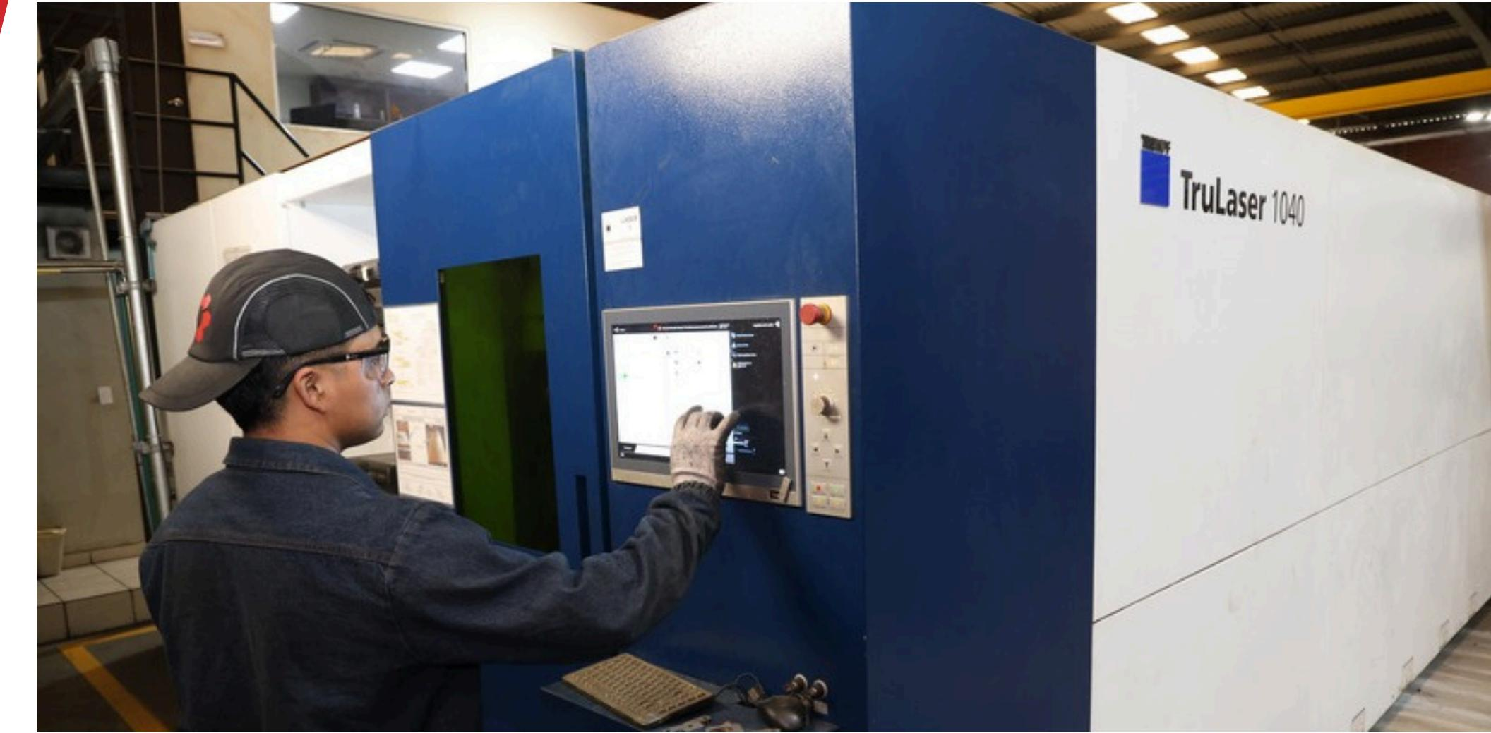
We use high-precision **TRUMPF** laser cutting technology for metal components ranging from 1 mm up to 1" in carbon steel, stainless steel, aluminum, and copper.
