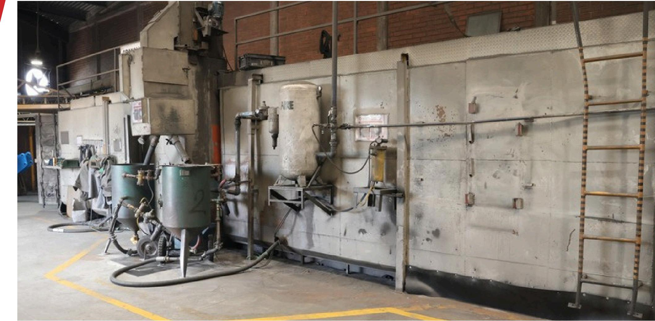
Our shot-blasting process ensures clean, uniform surfaces prepared to receive any type of coating. Through controlled abrasive blasting, we remove rust, scale, paint, and contaminants, achieving a consistent profile that enhances coating adhesion, extends service life, and elevates the final finish quality.
