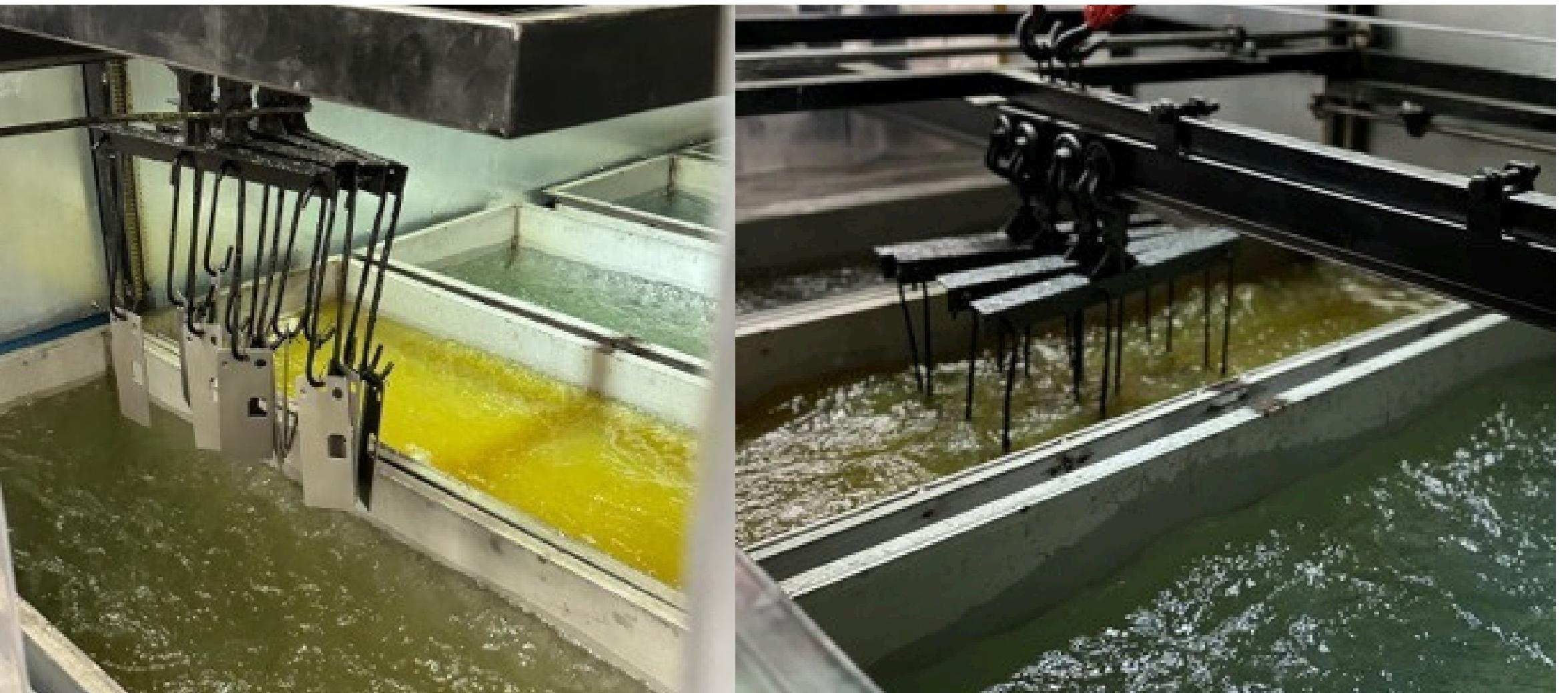
Zirconium pretreatment is an advanced surface preparation process that enhances coating adhesion and significantly improves corrosion resistance. Unlike traditional phosphate systems, zirconium provides a thinner, more uniform, and environmentally friendly layer, reducing water and chemical consumption without compromising performance.
